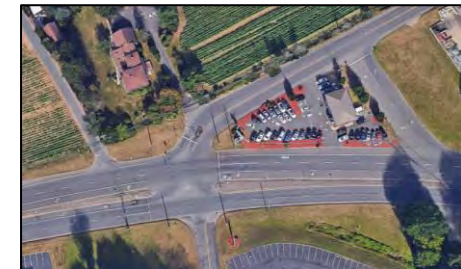
Close spacing between access to Wagner Ln and Main St
