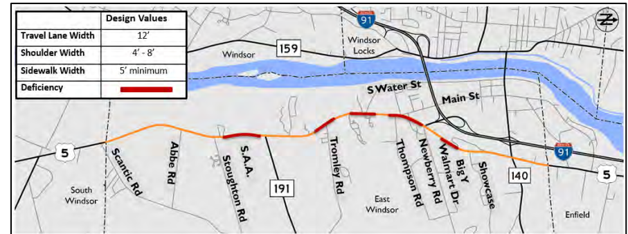
Figure 18: Locations of Deficient Shoulder Widths
