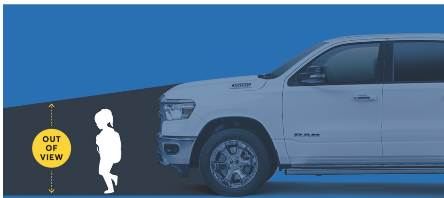
The hood heights of modern trucks can often obscure children and shorter adult pedestrians from the view of the driver. (Image: Consumer Reports, The Hidden Dangers of Big Trucks)
