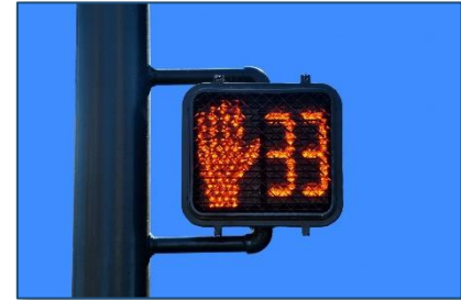
Figure 8: A crosswalk countdown signal showing the time left in a pedestrian crossing phase.
