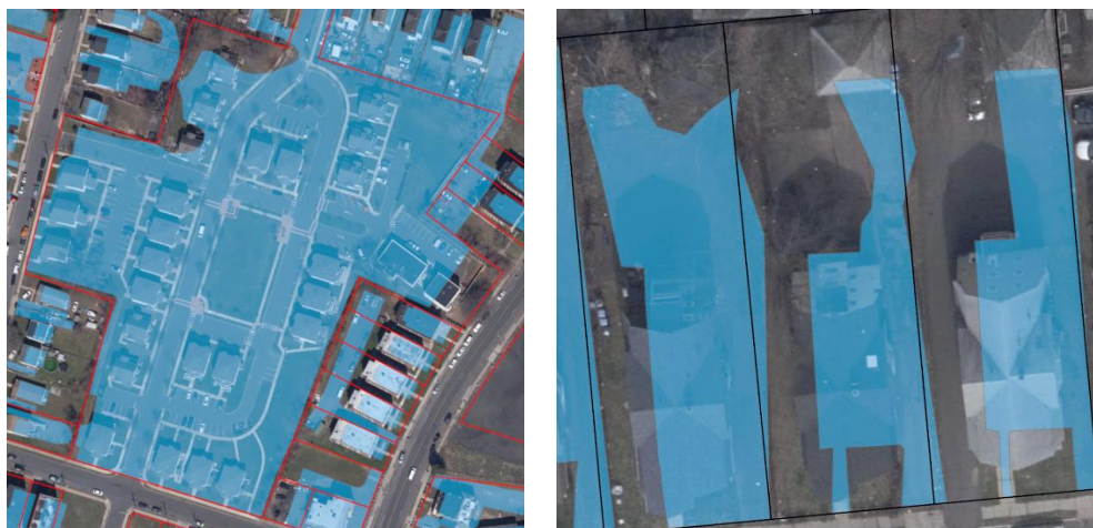
Figure 9. Examples of Missing IA and Over-Capture of IA
